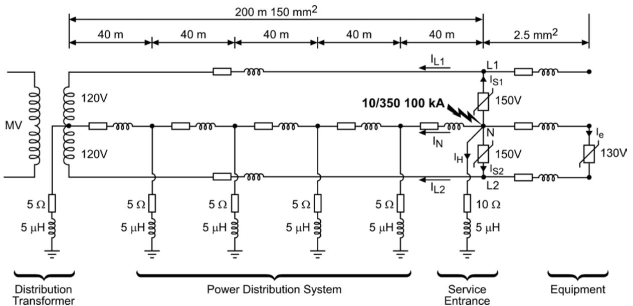
**Figure 1 Simplified building schematic with service-entrance SPDs, one built-in equipment SPD, and multiple-grounded power distribution system in case of a direct lightning flash to the earthing system**
